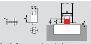
Calculating the necessary length of spindle extension:
